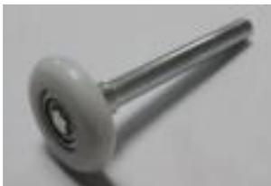
**ROLLERS:** Zinc-plated steel rollers with nylon roller and precision bearing designed to withstand a load of 60 kg at 750,000 revolutions.
